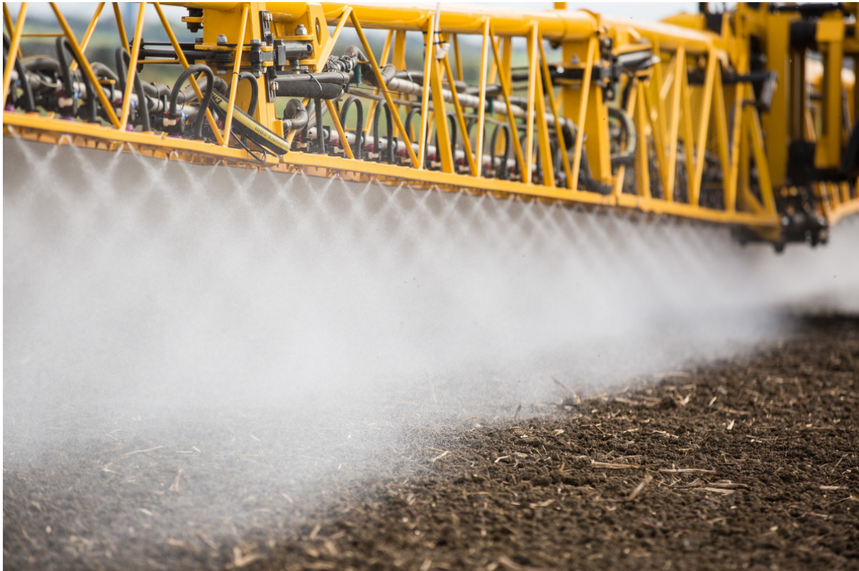
Herbizid im Einsatz (Foto: Chafer Machinery / flickr, Chafer Sentry, Applying Defy at 250l/ha on wheat land in Lincolnshire, bit.ly/29E6Sk4 , creativecommons.org/licenses/by/2.0 )
